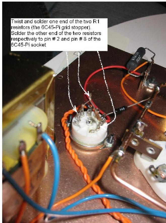
Figure 32. Wiring the grid stopper resistors (R<sub>1</sub>).
