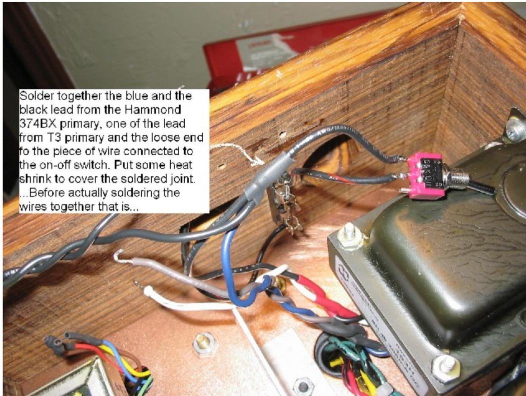
Figure 48. Final wiring of the on-off switch.
