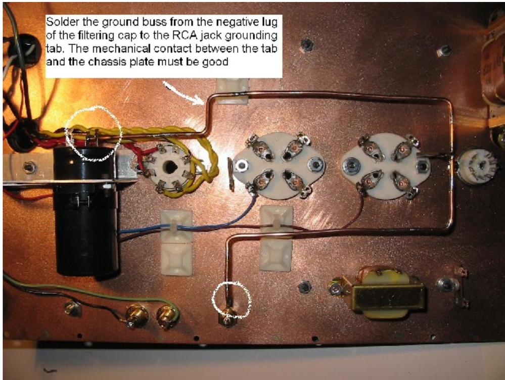
Figure 19. Overview of the ground buss location.
