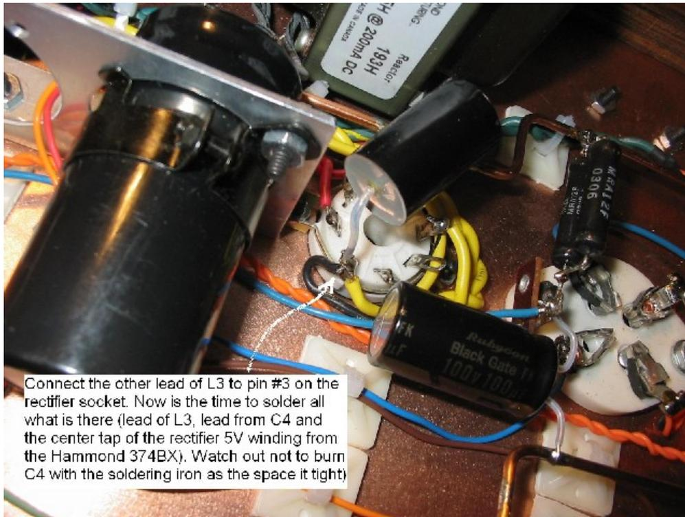
Figure 47. Final wiring of the rectifier socket.
