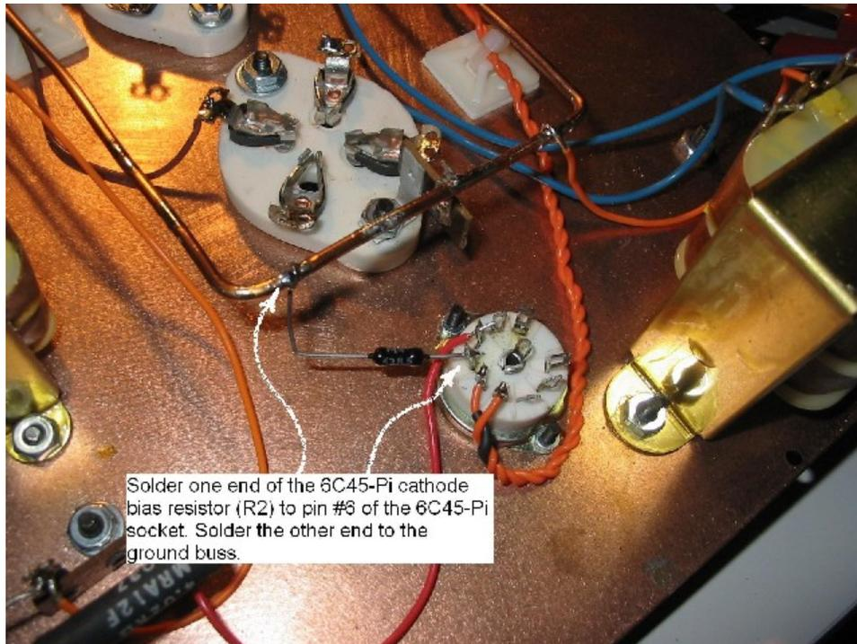
Figure 31. Wiring R<sub>2</sub>.
