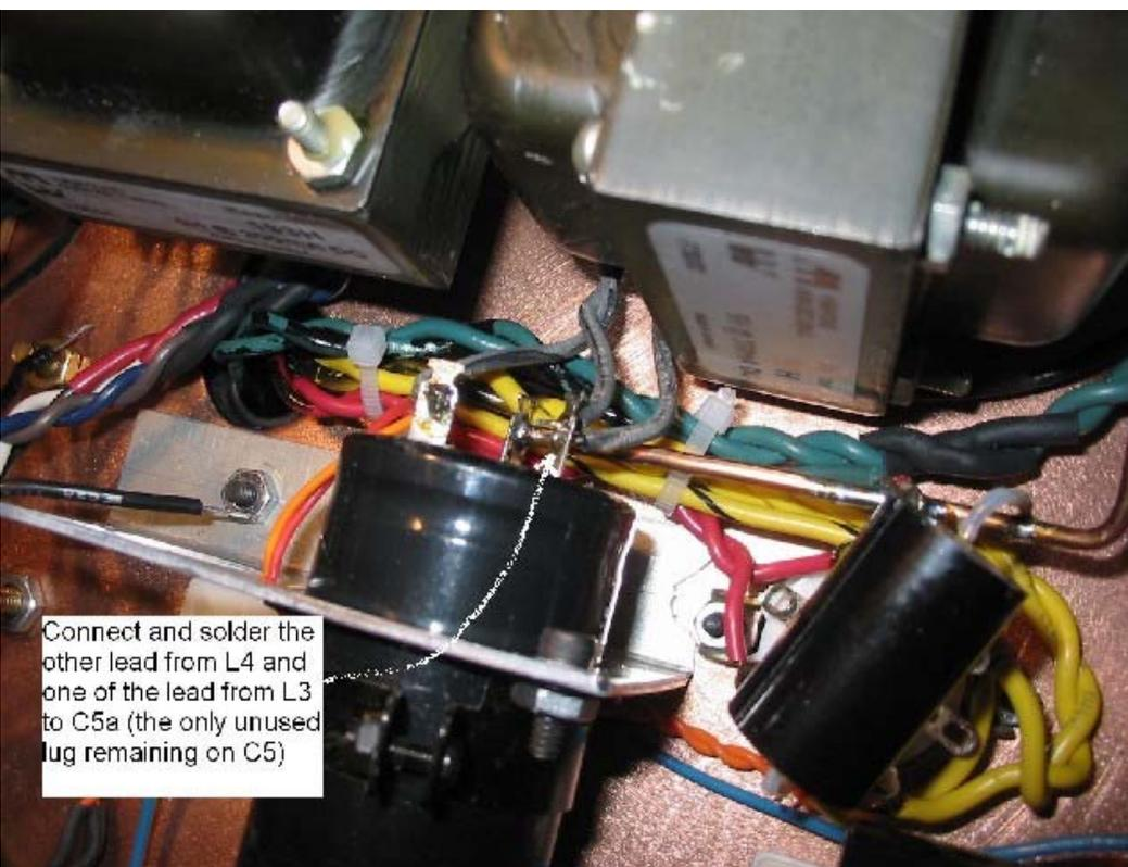
Connect and solder the other lead from L4 and one of the lead from L3 to C5a (the only unused lug remaining on C5)
