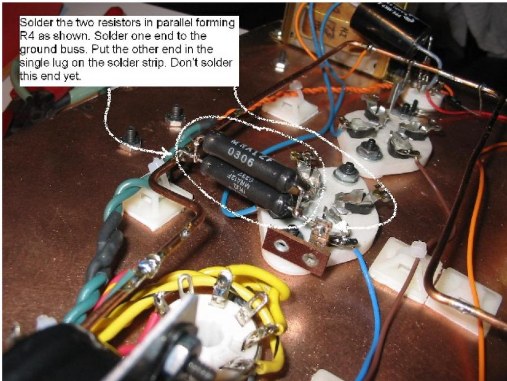
Figure 35. Installing R<sub>4</sub>.
