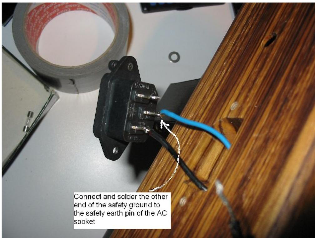
Figure 51. Wiring the safety ground (part 2).
