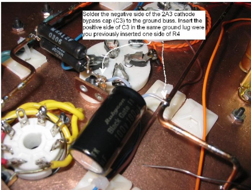
Figure 36. Installing C<sub>3</sub>.
