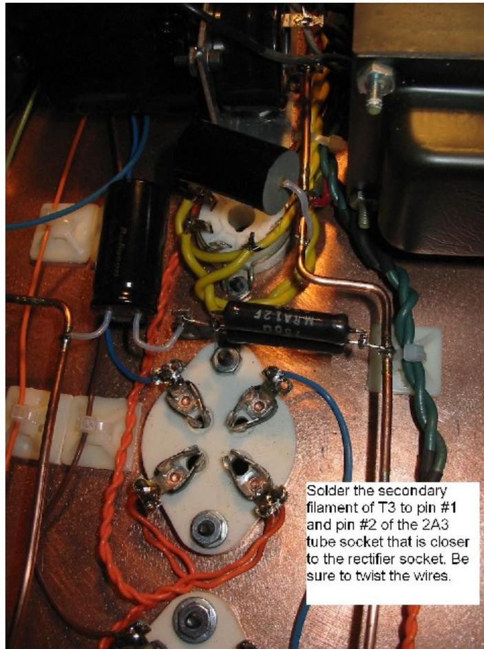
Figure 43. Soldering the secondary winding of T<sub>3</sub> to the rearmost 2A3 socket.
