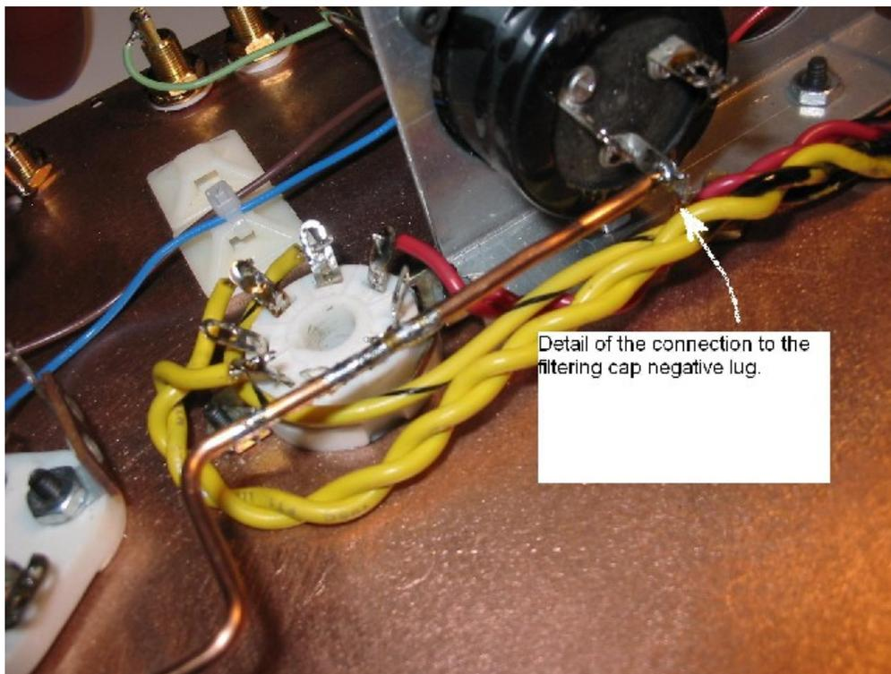
Figure 22. Detail of the ground buss connection to C<sub>5</sub> negative lug.
