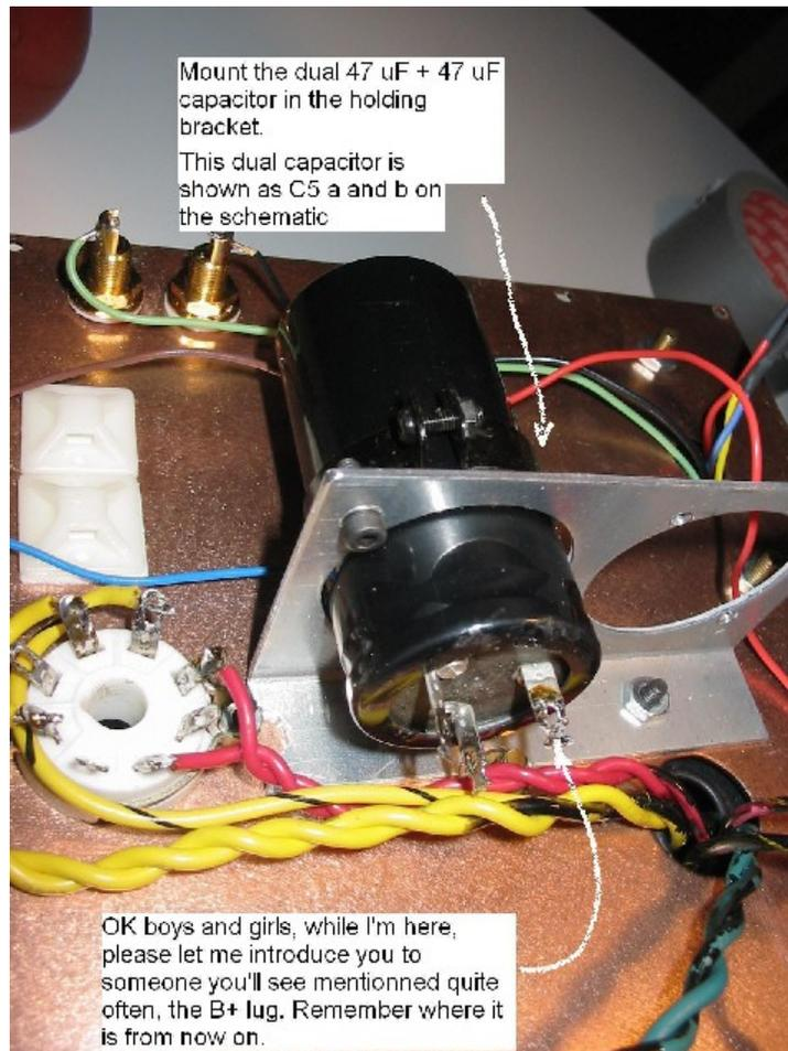
Figure 18. Installing  $C_5$ .
