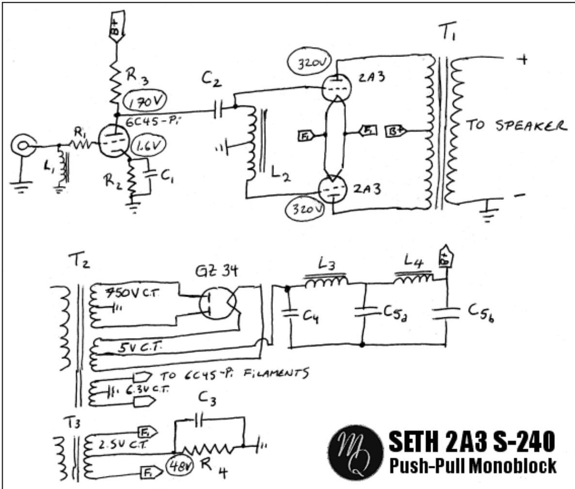
The rest of the amp is as simple. It is a two stage design where a 6C45-Pi drives a pair of 2A3 in push pull class A. The PSU is a double pi filter, making for a very low ripple. This amp is self biased. The pair of 2A3 shares a single bias resistor so this will ask for closely matched tubes. The list of the parts I used in these amps is given below. Feel free
