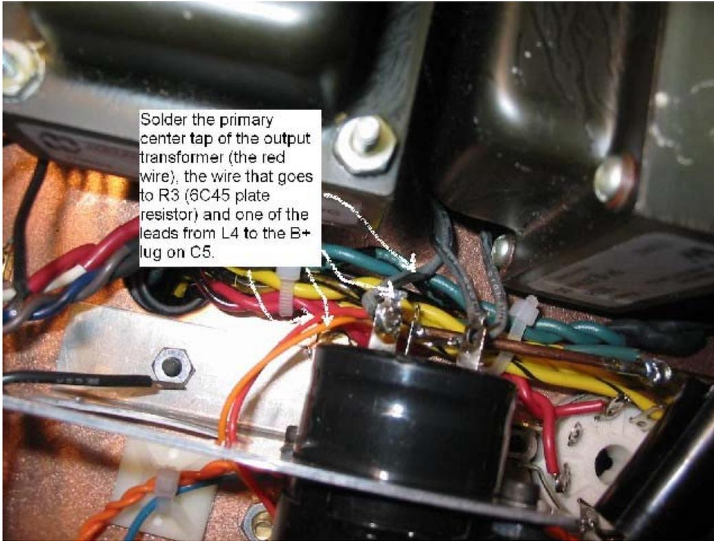
Solder the primary center tap of the output transformer (the red wire), the wire that goes to R3 (6C45 plate resistor) and one of the leads from L4 to the B+ lug on C5.
