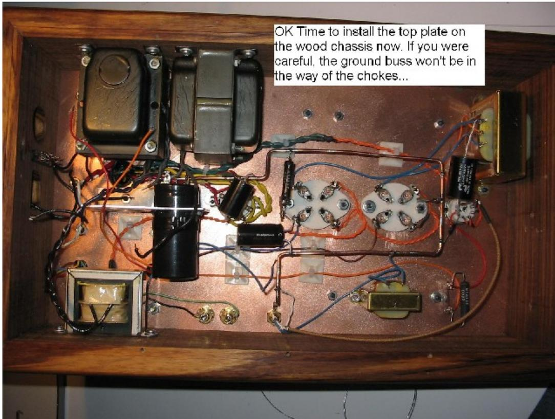
Figure 42. Installing the top plate on the chassis.
