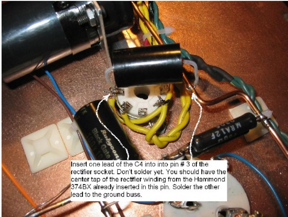
Figure 37. Wiring C<sub>4</sub>.
