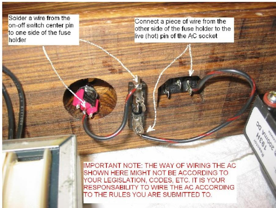
Figure 7. First step of the AC wiring
